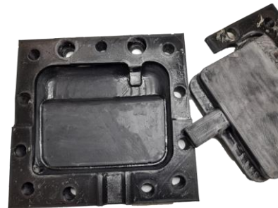
For complex pieces, Sterne proposes a silicone low-pressure molding technology in a 3D printed plastic mold.
