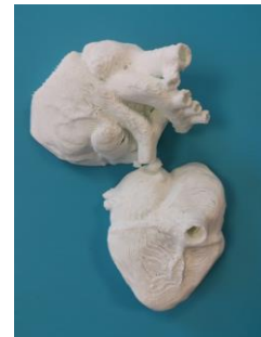
Heart printed using Sterne's 3D SiO-Shaping technique
